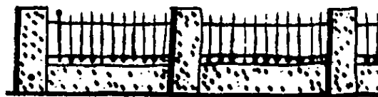
Low wall with masonry posts and articulated joints
