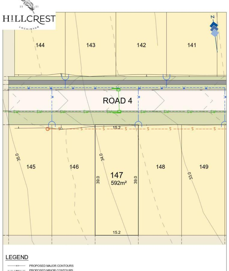
PROPOSED MINOR CONTOURS PROPOSED INTERALLOTMENT DRAINAGE PROPOSED SEWER LINE PROPOSED WATER MAIN 1:5 BATTER
