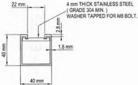
'ER-R-MT' RAIL DETAIL GRADE 6005-T5 ALUMINIUM ( SCALE 1:2 )
